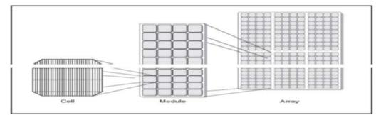
example of cells connected to form modules and modules connected for form arrays.
