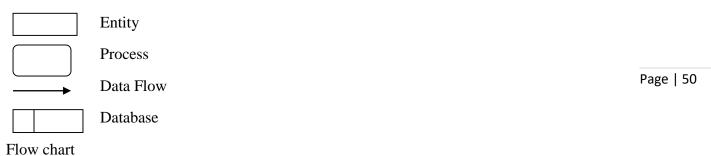
A flow chart is a graphical or symbolic representation of a process. Each step in the process is represented by a different symbol and contains a short description of the process step. The flow chart symbols are linked together with arrows showing the process flow direction. They are used to Define and analyze processes, build a step-by-step picture of the process for analysis, discussion, or communication and define, standardize or find areas for improvement in a process
