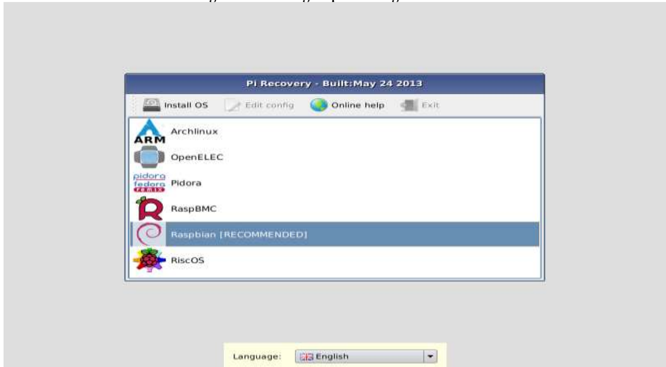
Figure 3: Installing raspbian using Noobs
